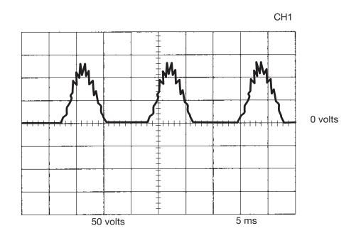
This is NOT the typical DC (+) output voltage waveform. One output diode is not functioning. Note the "gap" in the waveform. One output diode was disconnected to simulate an open or nonfunctioning output diode. Each vertical division represents 50 volts and each horizontal division represents 5 milliseconds in time.
